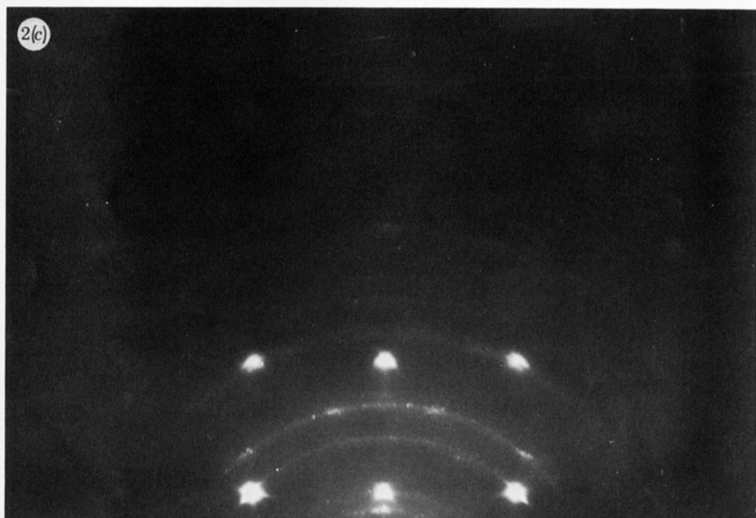
FIGURE 2. (a) Reflexion electron diffraction pattern (40 kV) from a \langle 100 \rangle gold film on KBr showing a mixture of rings from a thin overlayer plus short 'streaks' indicative of a stepped surface. (b) Scanning electron micrograph of a low r.r.r. \langle 100 \rangle gold film on KBr showing the grain size. (c) Reflexion electron diffraction pattern (40 kV) from a \langle 100 \rangle gold film showing faceted nature of grains as illustrated by diffraction 'stars'.
